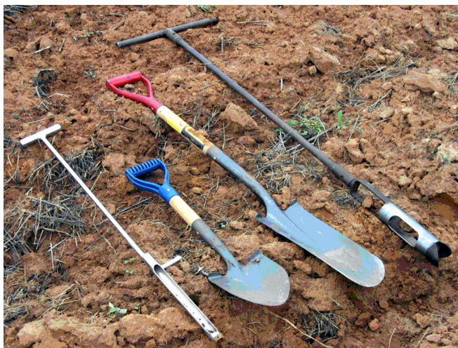
Figure 1. Examples of soil sampling equipment. From left, soil probe, spade, sharpshooter and soil auger.
