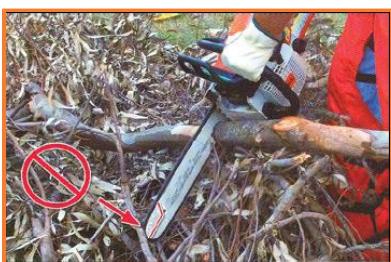
Figure 2. Do not cut with the upper tip!
