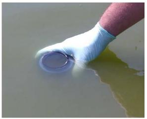
**Figure 3.** Seal under water to avoid trapping air
