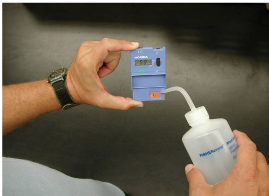
Figure 6. Hold meter vertically and gently wash tissue and sensor area off using de-ionized water from small water bottle with pointed tip.
