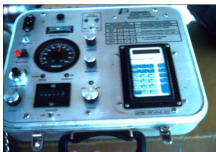
Figure 8. Transmitter and totalizing unit for ultrasonic flow meter.
