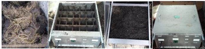
Figure 1. Sterilizing used potting medium in an electric Pro-Grow™ soil sterilizer.
