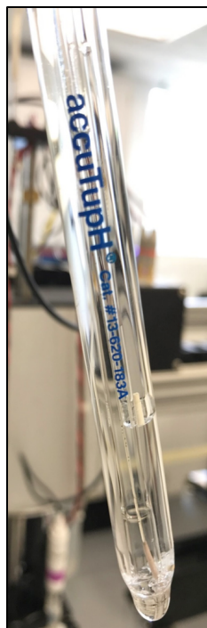
Figure 1. Combination glass pH electrode.
