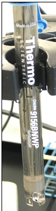
Figure 2. Combination epoxy pH electrode.
