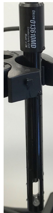
Figure 3. Graphite cell with 4-electrode-Epoxy sealed.
