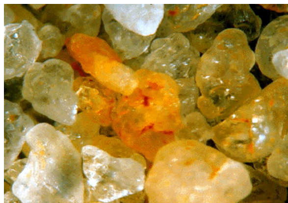
Figure 5. Close-up of coated sand particles. The coating is often a combination of clay and organic matter (reddish-brown material on sand grains), which greatly improves crop production on soils that have coatings.
