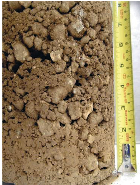
Figure 4. The profile of a gravelly soil. The soil is typical of soils found in the Homestead area, in the southern peninsula of Florida.
