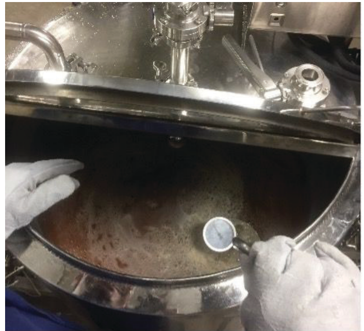
Figure 10. Boiling kettle filled with peach juice during sterilization. Credits: Savanna J. Curtis, former graduate student, UF/IFAS
