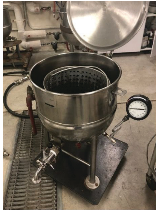
Figure 6. Boil-blanching steam kettle unit with a perforated basket inside used for transferring peaches to and from the kettle. Credits: Savanna J. Curtis, former graduate student, UF/IFAS
