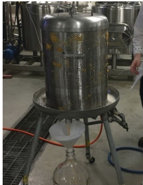
Figure 7. Standing basket bladder press during pressing operations. Credits: Andrew J. MacIntosh, UF/IFAS
