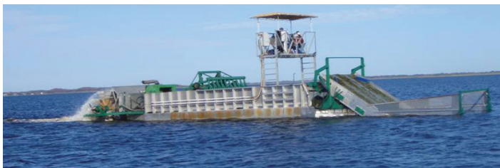
Figure 8. Mechanical harvester with hydraulically driven paddle wheels in the back and articulated cutter/conveyor tables in the front. Credits: James Leary, UF/IFAS Center for Aquatic and Invasive Plants
