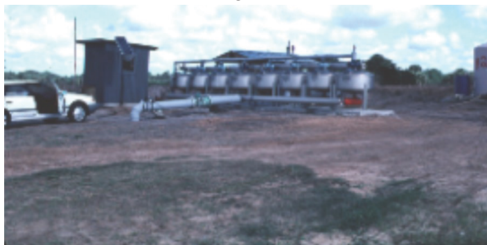
Figure 7. Media filters for filtering water used for drip irrigation of vegetables.
