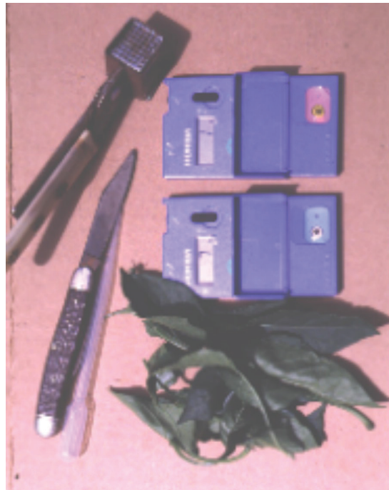
Figure 6. Ion-specific electrodes for measuring concentrations of nitrate-N and potassium in vegetable leaf petiole sap.
