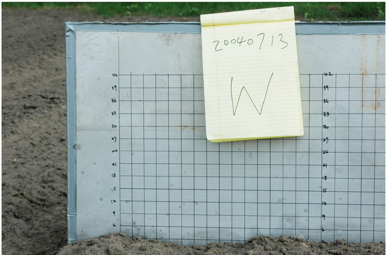
Figure A-84. Surface roughness measurement at the west side of footprint: across the row
