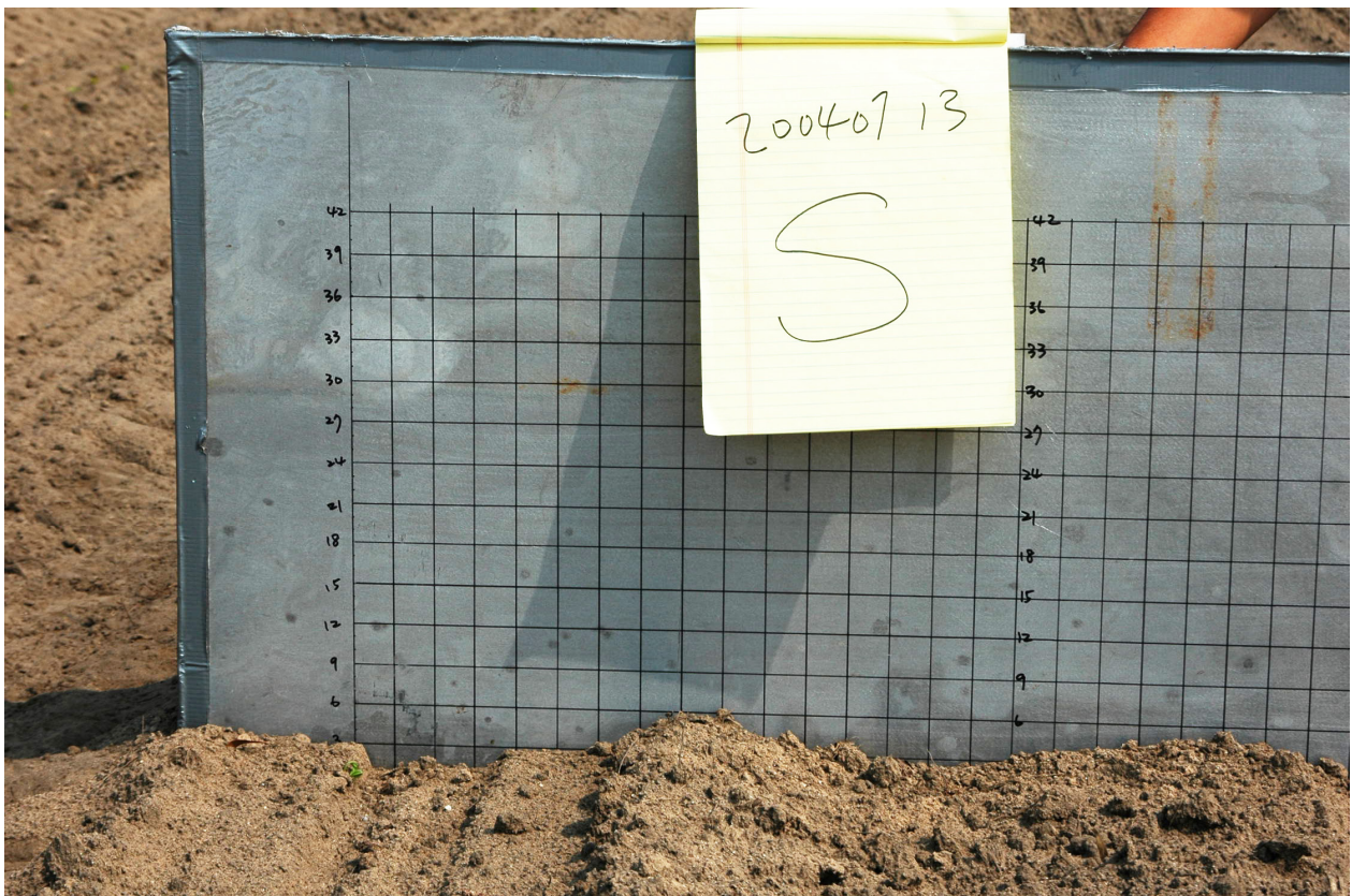
Figure A-82. Surface roughness measurement at the south side of footprint: across the row
