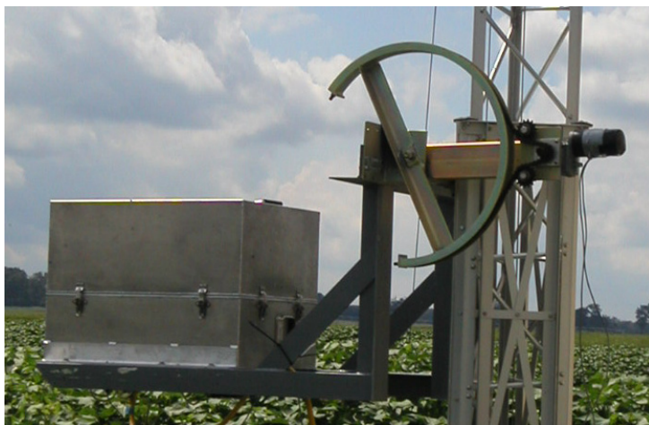
Figure 4 (b) and (c). The side view of the UFCMR showing the rotary system and the front view of the UFCMR showing the receiver antenna.
