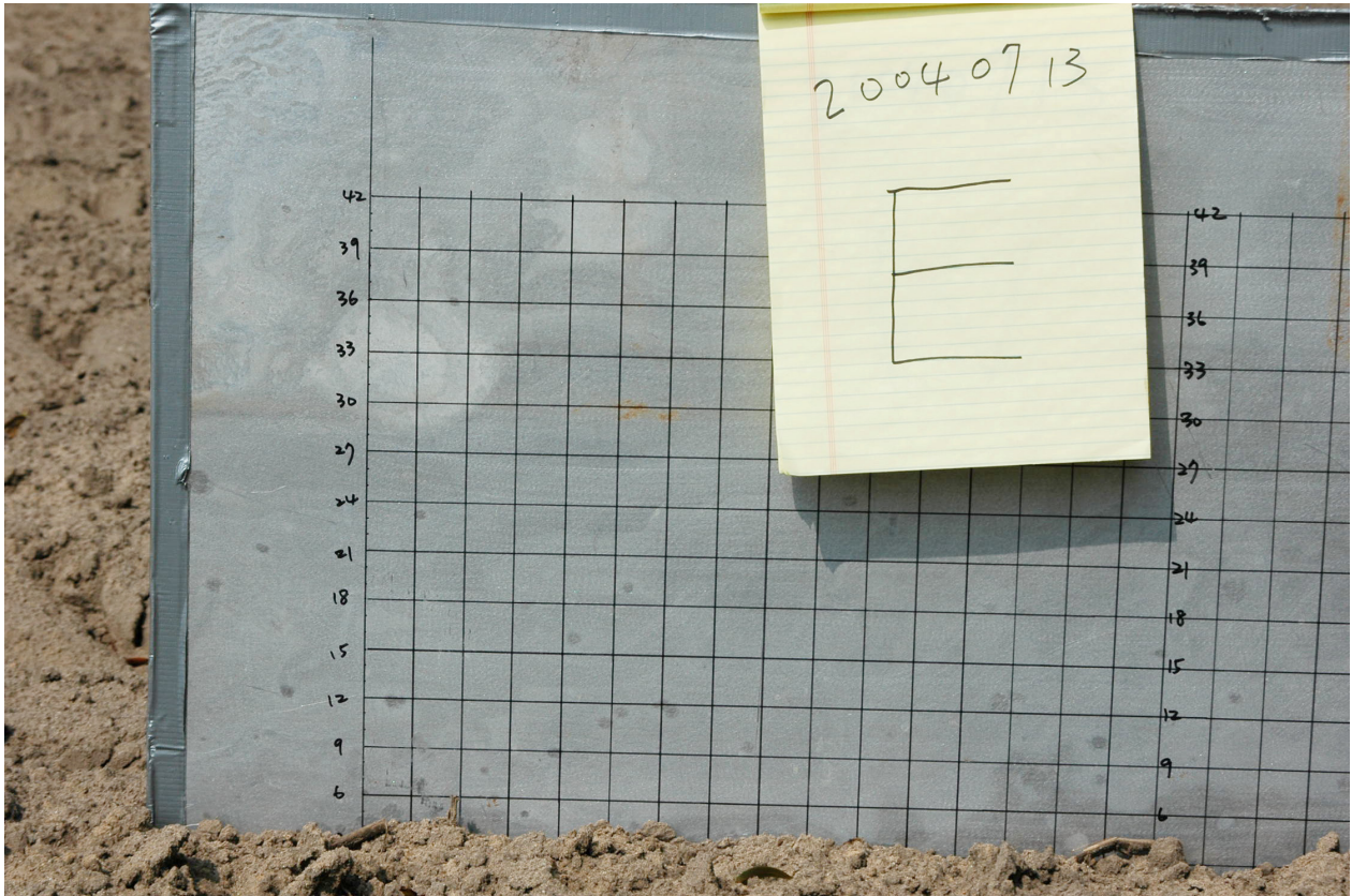
Figure A-79. Surface roughness measurement at the east side of footprint: along the row
