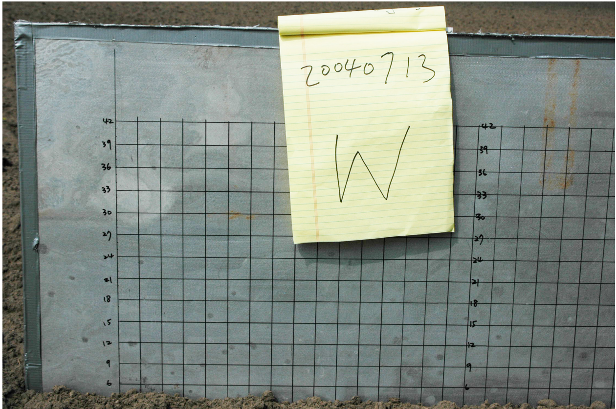
Figure A-83. Surface roughness measurement at the west side of footprint: along the row
