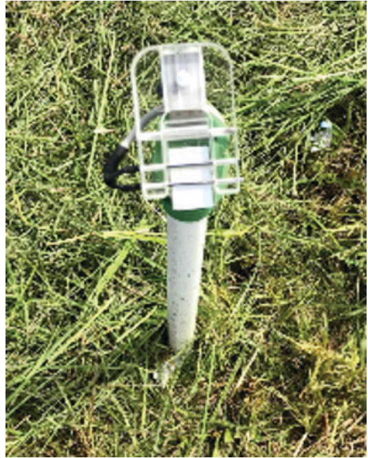
Figure 8. Paper-based LWS with paper in good condition. Credits: T. B. Onofre, UF/IFAS
