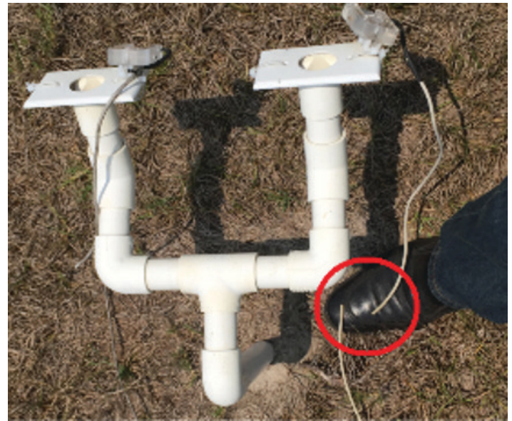
Figure 11. Leaf wetness sensor with cable damaged. Credits: T. B. Onofre, UF/IFAS
