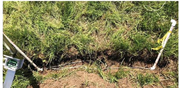
Figure 12. Preparation to bury and protect a leaf wetness sensor's cable. Credits: T. B. Onofre, UF/IFAS
