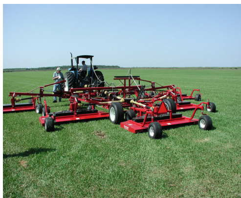
Figure 6. Sod mower with a 36-foot swath.
