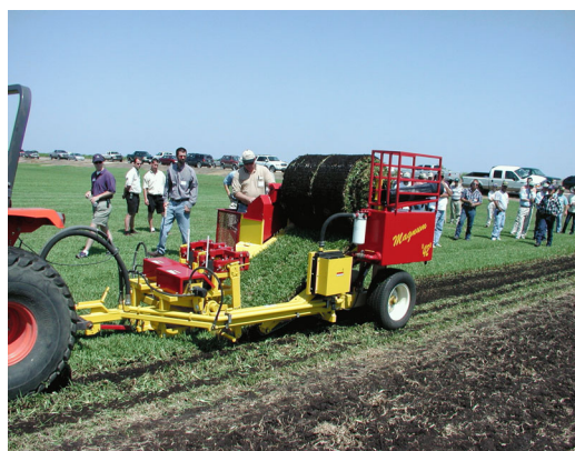
Figure 7. Cutting rolls for landscape use with a sod harvester.
