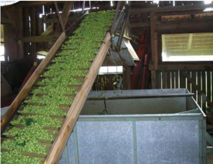
Figure 6. Picked and sorted hops at the end of the picking machine. Credits: Public domain, Wikimedia Commons
