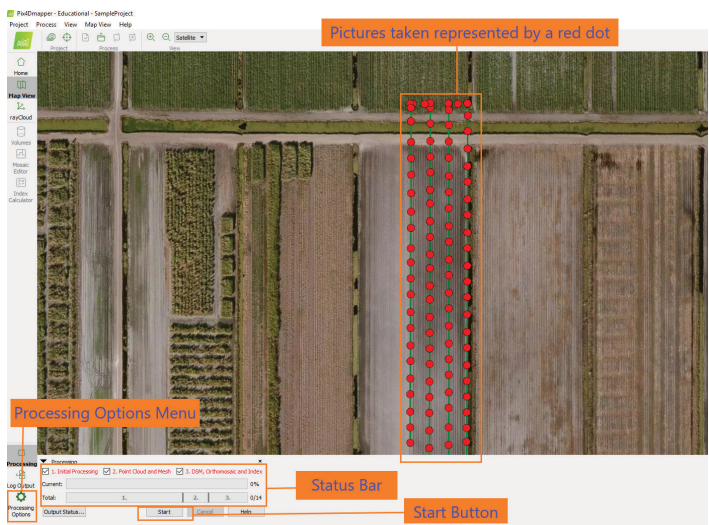
Figure 5. Screenshot of Pix4Dmapper window showing the collected data, processing options menu, status bar, and start button. Credits: UF/IFAS
