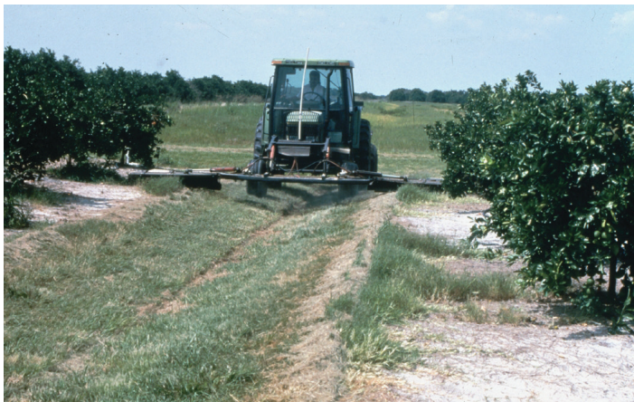
Figure 4. Boom applicator used to apply suspension fertilizers. Credits: Stephen Futch, UF/IFAS
