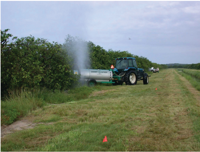
Figure 5. Airblast sprayer used to apply soluble nutrients to citrus tree foliage.
