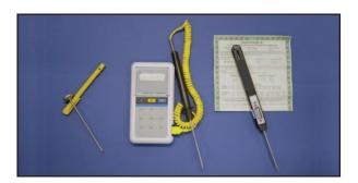
The method and frequency of calibration for thermometers will depend on the use and temperature range where the equipment is used. In the absence of manufacture's recommendations, thermometers should be calibrated at least once a month with more frequent calibrations when the instrument is physically abused or if the readings are questionable.
