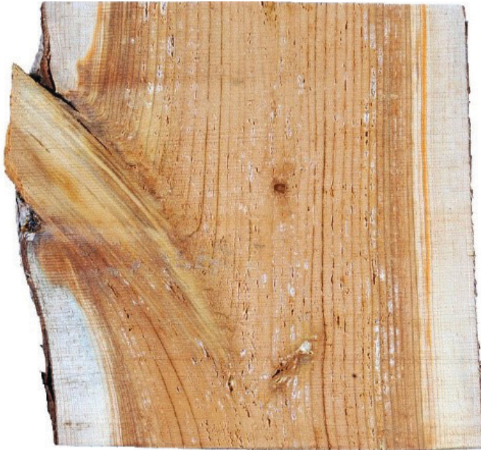
Figure 1. Symptom of red heart disease caused by Porodaedalea pini , showing the reddish-brown decay with “white pocket” in the heartwood.
