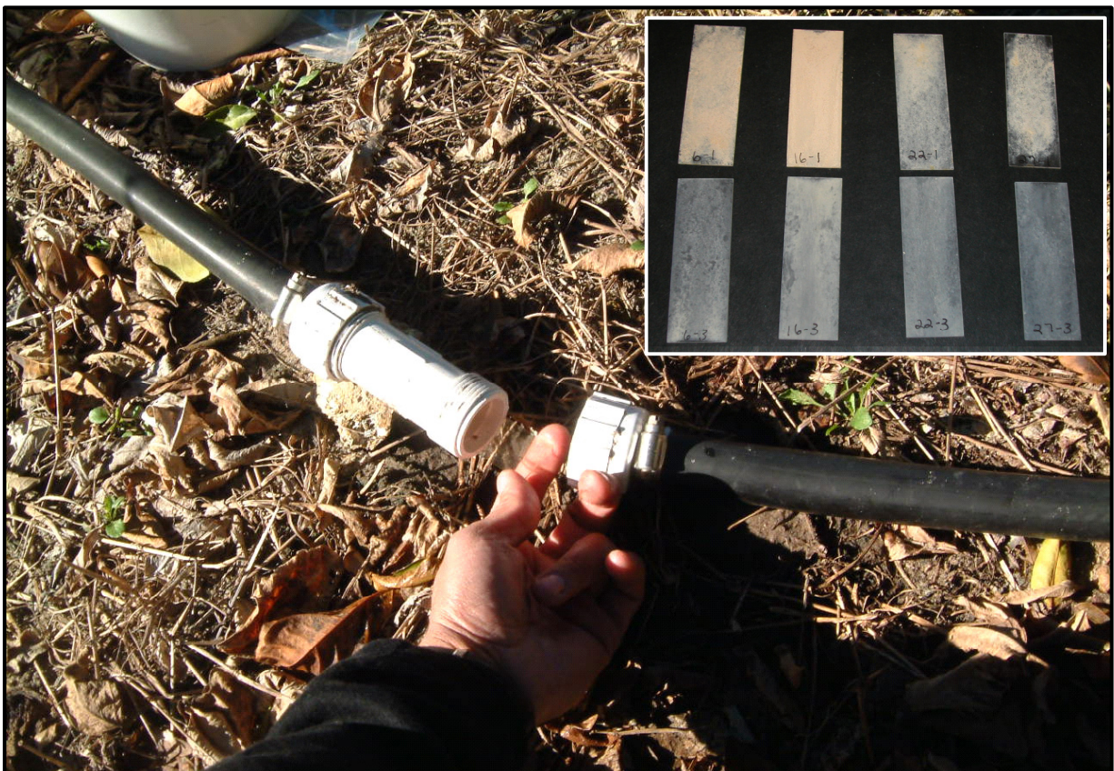
Fig. 3. A \frac{3}{4} -inch PVC coupling found in plumbing-supply stores can serve as an in-line glass slide holder. Observing the amount, type, and rate of scale deposition occurring on a clean slide (inset) can help determine the scaling potential of the irrigation water and the effect of injected scale-inhibiting chemicals.
