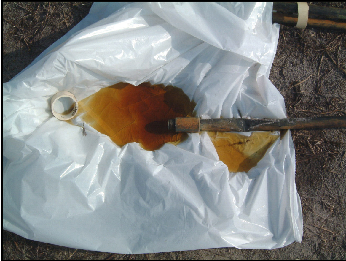
Fig. 6. The reddish-brown color of the flush water from an iron-scaled microirrigation system purged with 1% citric acid suggests that the acid dissolved the scale.
