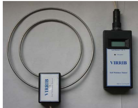
Figure 7. Phase transmission probe.
