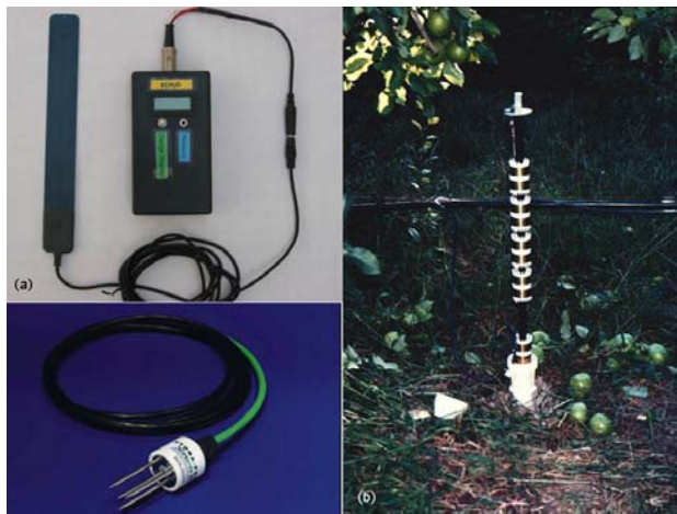
Figure 5. FD probes: a) Capacitance (plates imbedded in a silicon board); b) Capacitance (rods); and c) FDR (rings).
