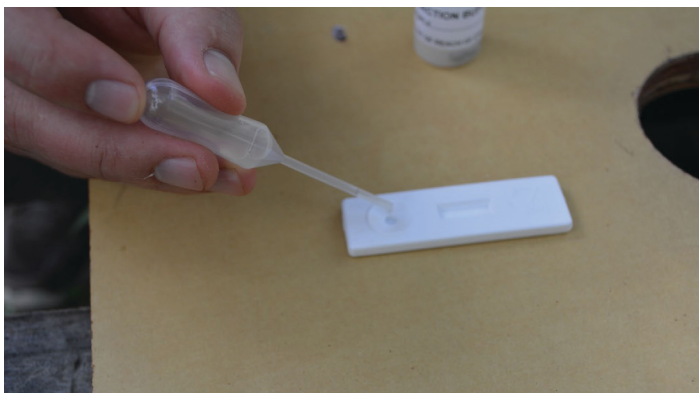
Figure 10. Squeezing two drops of the sample into the sample well with the pipette. Credits: C. Mueller, UF/IFAS Honey Bee Lab
