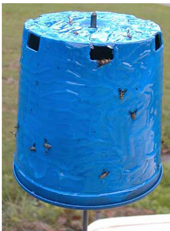
Figure 12. A blue colored cylinder covered with sticky material makes an effective removal trap for deer flies and other tabanids when attached to a slow moving object (< 7 mi/hr). Credits: R. F. Mizell, III, University of Florida
