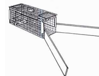
Figure 3. A live-trap with "wings" added to help guide the armadillo into the trap (Reprinted from Prevention and Control of Wildlife Damage by University of Nebraska, USDA-APHIS, and the Great Plains Agricultural Council).
