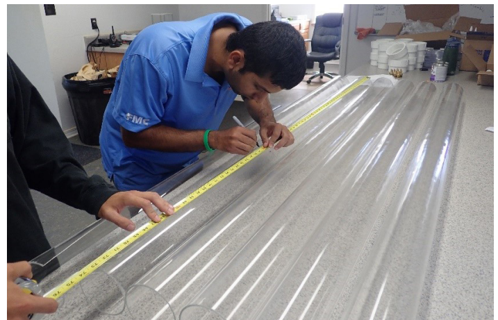
Figure 3. Clear acrylic tubes to be cut at 4-ft lengths. Credits: Cropping System Lab, UF/IFAS
