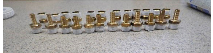
Figure 18. Teflon tape added to \frac{1}{2} -inch brass male adapter and \frac{3}{8} - \frac{1}{2} -inch capacity brass barb.
