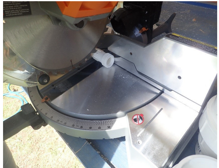
Figure 8. ½-inch repair coupling is cut in half.
