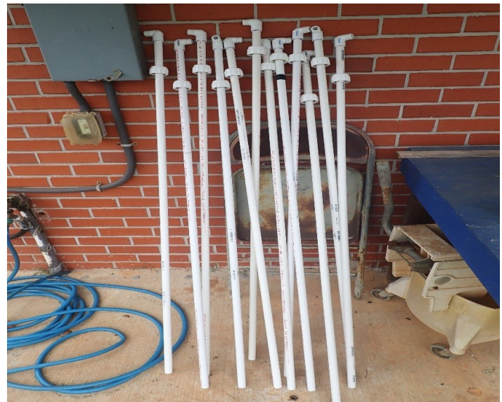
Figure 24. Air tube with the cap of repair coupling, rubber stopper/gasket, and elbows assembled. Credits: Cropping System Lab, UF/IFAS
