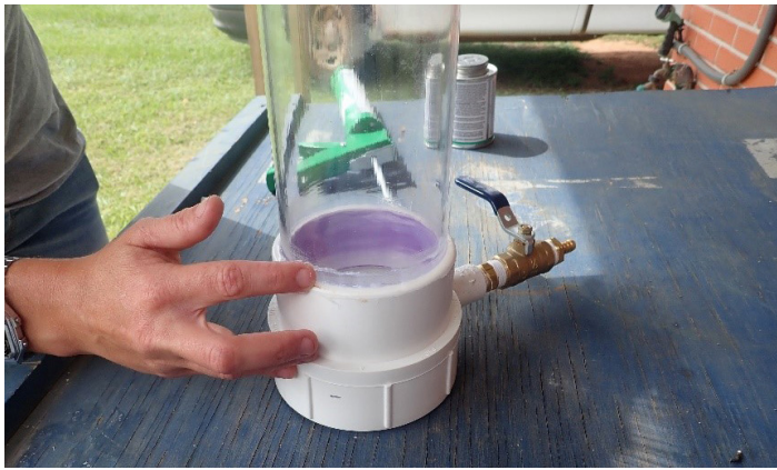
Figure 26. Silicone is applied at the top and bottom ends. Credits: Cropping System Lab, UF/IFAS
