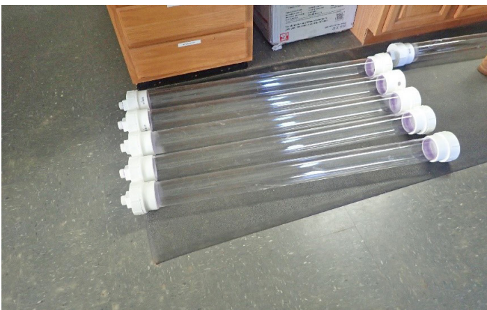
Figure 17. Siphon in the making, showing the acrylic tube, top (left) and bottom (right) ends.
