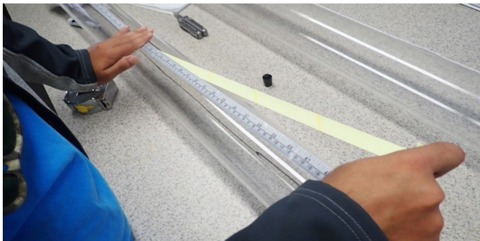
Figure 27. An adhesive tape measure is glued to the siphon to facilitate reading of the water level during measurement. Credits: Cropping System Lab, UF/IFAS
