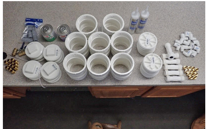
Figure 2. Assembly of fittings for the construction of multiple siphons. Credits: Cropping System Lab, UF/IFAS
