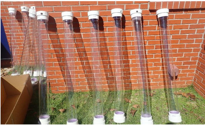
Figure 15. Acrylic tubes with fixed top and bottom slip thread adapters.
