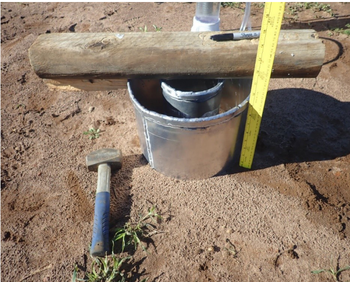
Figure 5. Double rings are hammered into the ground using a hammer and a piece of wood. Credits: Cropping System Lab, UF/IFAS
