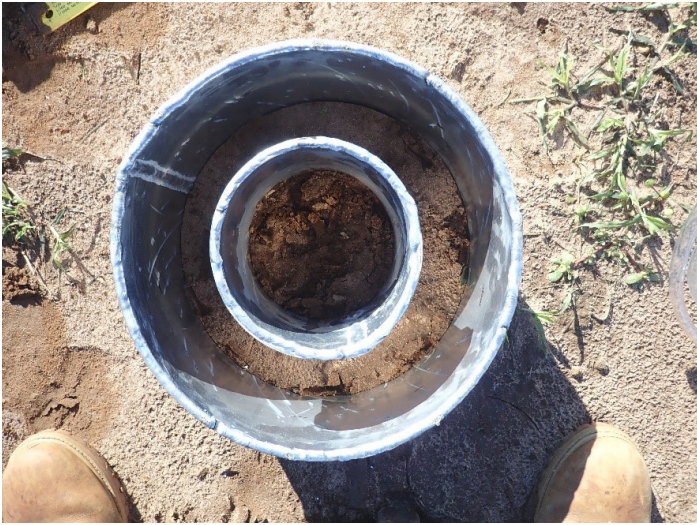
Figure 4. Concentric double rings deployed in the field to prevent lateral water movement from the inner ring. Credits: Cropping System Lab, UF/IFAS
