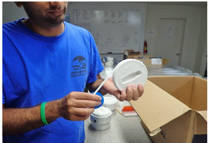
Figure 13. Teflon tape is added to the threaded PVC cap for the bottom of the siphon.
