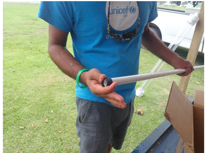
Figure 23. Rubber gasket used to create airtight seal at the top end of the siphon. Credits: Cropping System Lab, UF/IFAS
