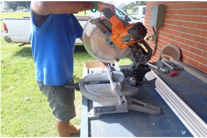
Figure 21. ½-inch air tube cut to a length of 57 inches. Credits: Cropping System Lab, UF/IFAS
