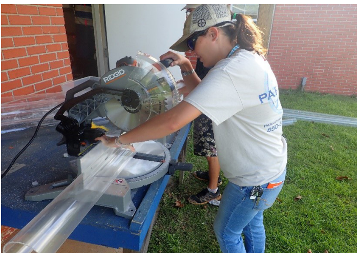
Figure 6. Acrylic tubes cut to 4 ft. Credits: Cropping System Lab, UF/IFAS
