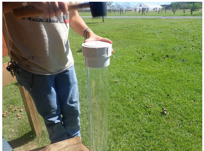
Figure 14. The bottom end of the siphon is glued and hammered into the acrylic tube with a rubber mallet.
