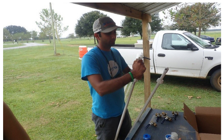
Figure 25. ½-inch brass ball valve screwed onto elbow at the top of the air tube. Credits: Cropping System Lab, UF/IFAS
