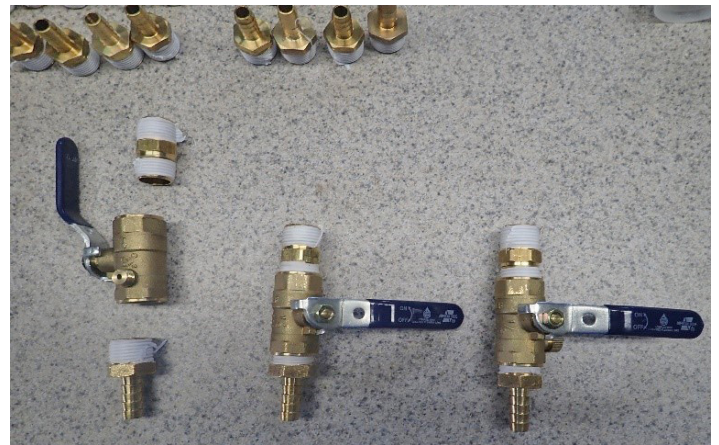
Figure 19. Assembling \frac{1}{2} -inch brass male adapter, \frac{1}{2} -inch brass ball valve, and brass barb with \frac{3}{8} - \frac{1}{2} -inch capacity.
