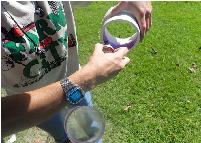
Figure 11. A 4-inch slip thread adapter is glued to the top of the clear acrylic tube and is later hammered into place with a rubber mallet for the bottom of the siphon.
