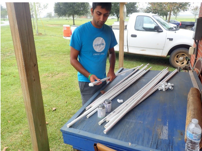
Figure 22. Elbow fitted to the air tube with primer and PVC glue. Credits: Cropping System Lab, UF/IFAS
