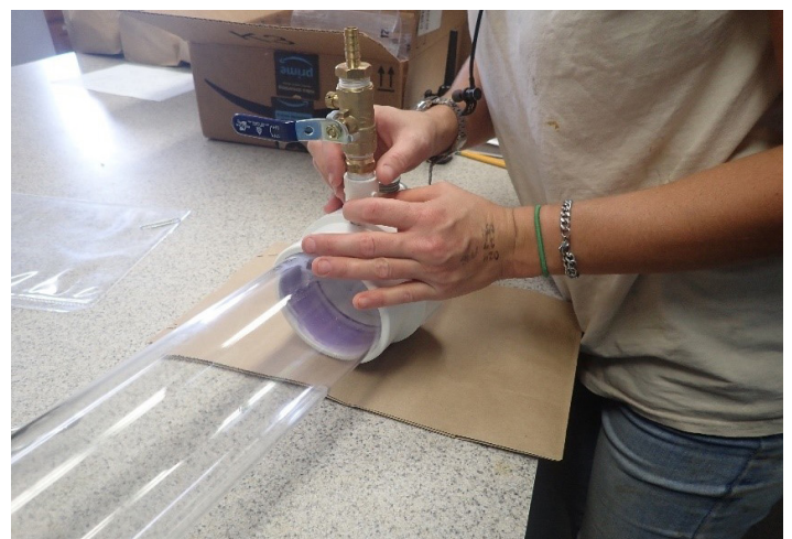
Figure 20. Assembled outlet port (riser, male adapter, brass ball valve, and brass barb) glued into bottom slip thread adapter.
