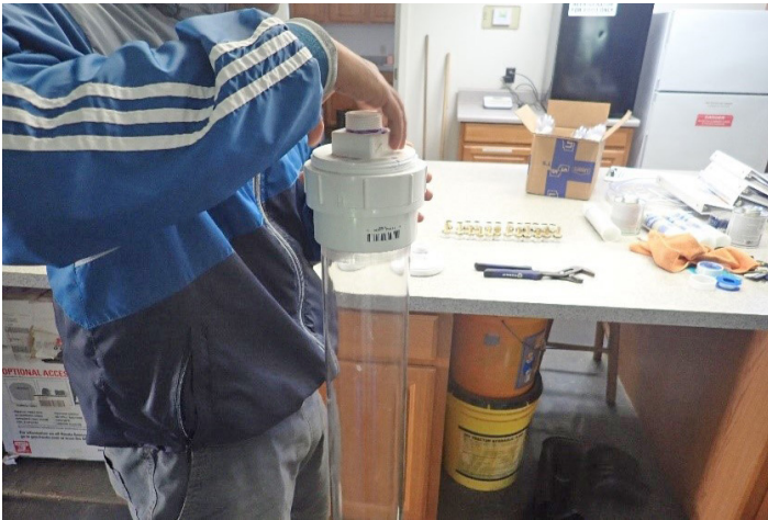
Figure 16. Assembled threaded cap is screwed into the 4-inch slip thread adapter for the top.
