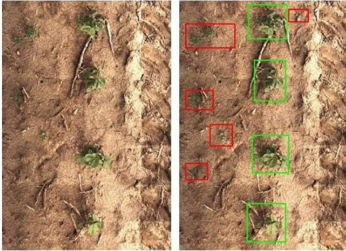
Figure 1. Plant and weed detection using computer vision and AI. Credits: Blue River Technology
