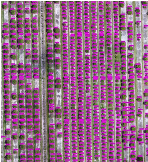
Figure 5. Citrus tree detection and counting (97% overall accuracy) using AI-based algorithms. Original picture taken by an unmanned aerial vehicle (UAV). Credits: UF/IFAS
