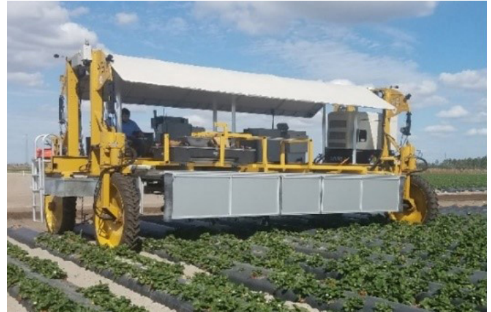
Figure 3. Harvest CROO Robotics (HCR) strawberry harvester. Credits: UF/IFAS
