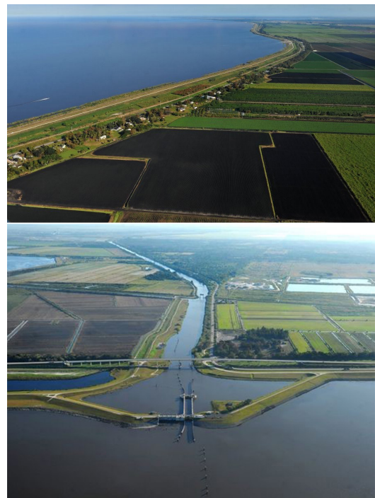
Figure 2. The Herbert Hoover Dike (above left) now surrounds Lake Okeechobee, except for an area on the west side where water flows into the lake from Fisheating Creek. Water control structures, (above right) move water into or out of the lake.
