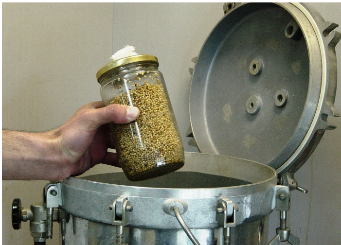
Figure 5. Sterilized seeds in a glass jar with a cotton plug to allow air exchange; ready for inoculation. Credits: Khalid Hammeed
