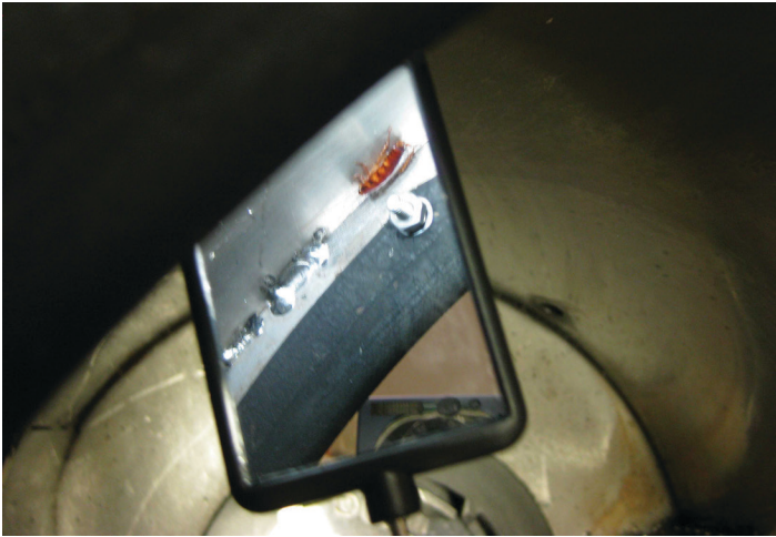
Figure 5. Use an inspection mirror and flashlight to help you see under and around areas that are difficult to reach. Inspection mirrors can be found in any hardware or auto mechanic store.
