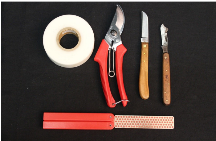
Figure 4. Budding tools. From left to right: budding tape, hand pruner, budding knives. Bottom: sharpening stone. Credits: Thang Kim, UF/IFAS
