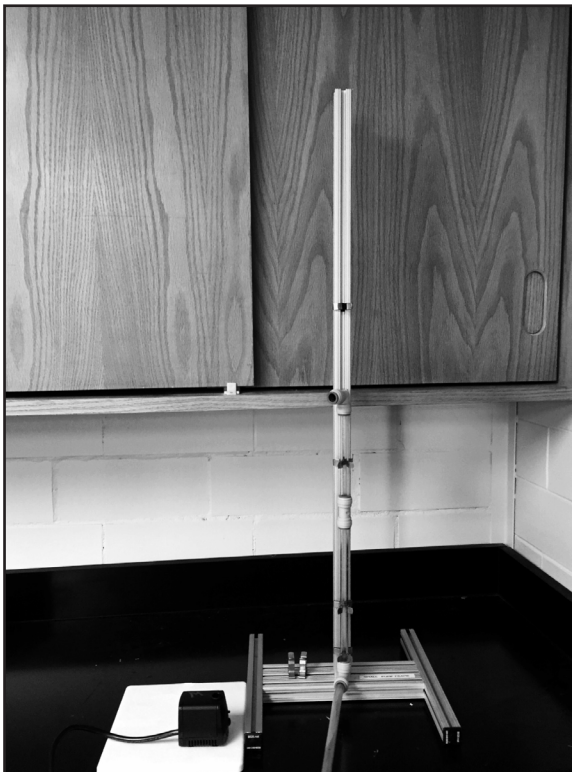
Figure 2. The frame used for the centrifugal pump experiments. One submersible centrifugal pump is on the left. It was placed in a container of the fluid during the experiments.
