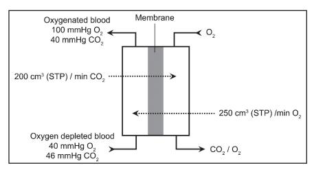
**Figure 3.** Membrane with gas transfer and concentration (partial pressures) values. As in the lungs, carbon dioxide is not completely removed to prevent alkalosis.<sup>[18]</sup>
