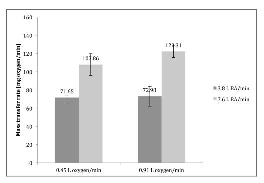
**Figure 7.** Mass transfer rates for all four operating conditions listed in Table 3 showing standard error of mean values. Each value is an average of gas side and liquid side mass transfer rates based on three trials. Error bars are standard error. The overlapping standard error bars allow students to conclude that the difference between means is significant, and therefore the oxygen flow rate does not have an effect on the mass transfer rate under these conditions.
