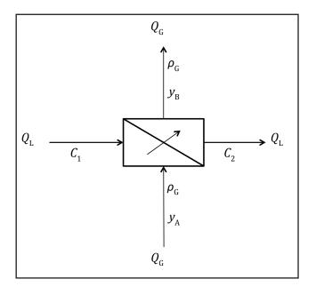
Figure 5. Blood oxygenator labeled with variables used in Eq. (3). Arrow in the center indicates oxygen mass transfer across membrane, which may be calculated using Eqs. (1) and (2) for the liquid side and gas side, respectively.
