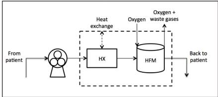
Figure 2. Unit operations in a heart-lung machine. Gas transfer is accomplished via membrane oxygenators, which have largely supplanted the bubble oxygenators used in early cardiopulmonary bypass (CPB) systems.<sup>[17]</sup> Heat exchange (HX) is required to maintain the desired body temperature. Heat exchanger and membrane are commonly combined into a single, disposable unit.<sup>[13]</sup>
