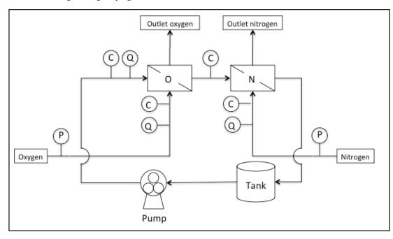
Figure 4. The blood oxygenator testing system showing the two hollow fiber membrane modules used for gas exchange (Module O oxygenates the blood analog; Module N deoxygenates the blood analog). Concentration (C) measurements are taken at the inlet and the outlet of each hollow fiber membrane module. Gas pressure (P) is measured on the oxygen and nitrogen inlet streams, and liquid flow rate (Q) is measured on the blood analog inlet stream.
