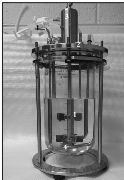
Figure 4. Bioreactor (New Brunswick Bioflo reactor, model 115) [16] where 1 is the dual flat blade impeller, 2 is the head plate which holds the pH, temperature and dissolved oxygen probes, 3 is the impeller motor, and 4 is the air sparger.
