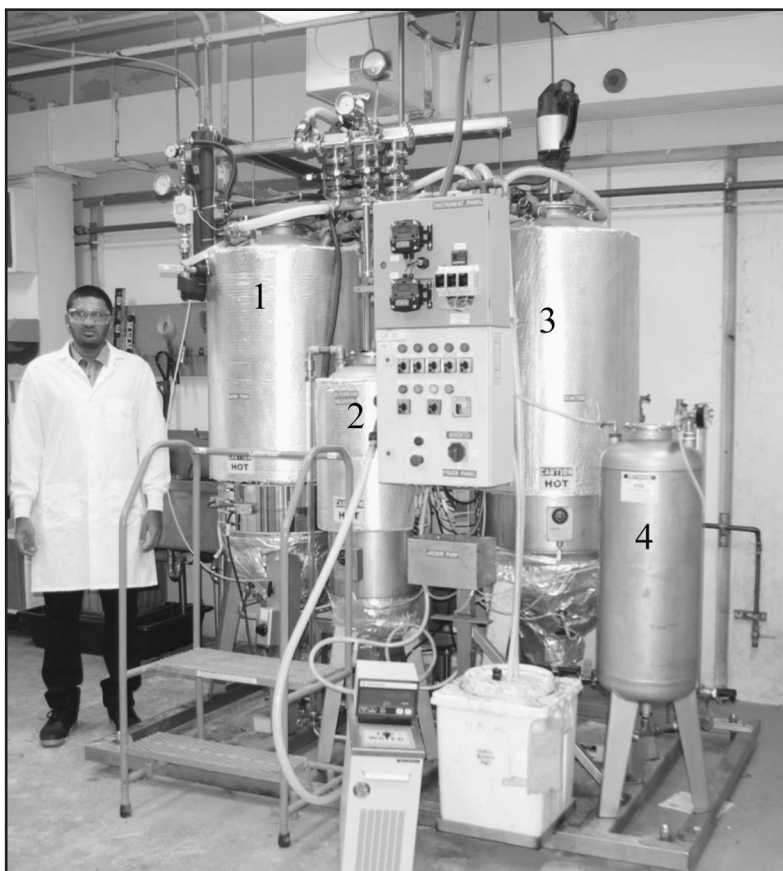
Figure 5. Pilot plant scale biodiesel processor, where 1 is the wash tank, 2 is the catalyst recovery tank, 3 is the reactor and 4 is the methanol recovery tank; catalyst tank and methanol tank are located on the back side of the processor (not shown). Student pictured is Chirag Mevawala.
