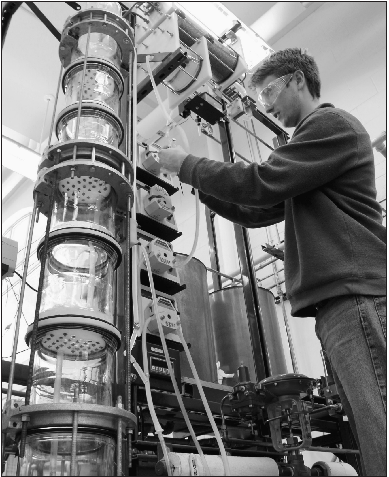
Student McLain Leonard works on a trayed distillation column in the teaching lab.
