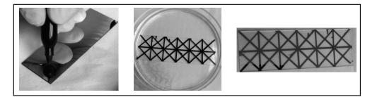
Figure 4. Copper electrode fabrication. The desired design was first drawn on a coppercoated glass slide with a permanent marker. Unwanted copper was etched away in a 3:1 mixture of 3% H<sub>2</sub>O<sub>2</sub> and 10 M HCl. To reveal the final copper electrodes, the permanent ink was washed away with acetone.
