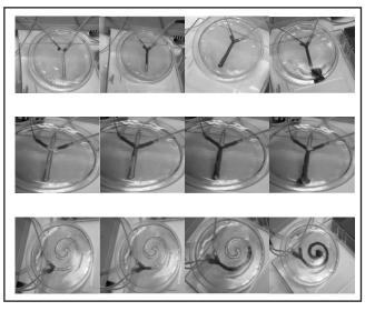
Figure 2. Fluid mixing on different gelatin chips. Red food color, milk, and blue food color were used for better visualization, as shown in different grayscale shades. The channel cross section was 3 mm by 2 mm (W x H).
