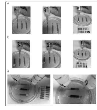
Figure 3. Homemade pH sensor for acid and base detection. (a) 0.1 M HCl. (b) 0.1 M NaOH. (c) Neutralization test. The acid and base were loaded at the same time from the two ends of a channel. The test strip showed three grayscale shades, corresponding to different pH values.
