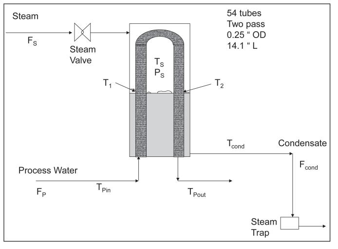
kg/s). So the sensible heat removed from the liquid in the bottom of the heater can be calculated.
