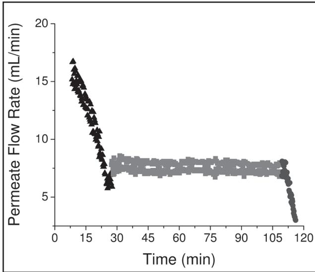
**Figure 6.** The three stages of diafiltration: first concentration step (▲), diafiltration step (■), and the second concentration step (●). The diafiltration process is run at a feed flow rate of 300 mL/min and at a TMP of 20 psi.
