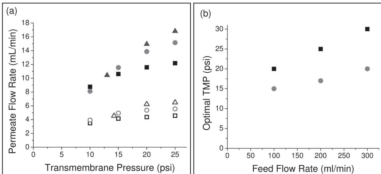
**Figures 4.** a) TMP Optimization for BSA concentrations of 9.59 mg/mL (solid symbols) and 65.9 mg/mL (open symbols) at various feed flow rates ( $Q_{feed} = \blacksquare$  100 mL/min |  $\bullet$  200 mL/min |  $\blacktriangle$  300 mL/min).
