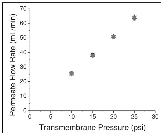
**Figure 3.** The results of the water permeability test demonstrate that the permeate flow rate is linearly dependent on  $P_{TMP}$  and independent of the feed flow rate. ( $Q_{feed}$  = ■ 50 mL/min | ● 150 mL/min | ▲ 250 mL/min | ▼ 300 mL/min).
