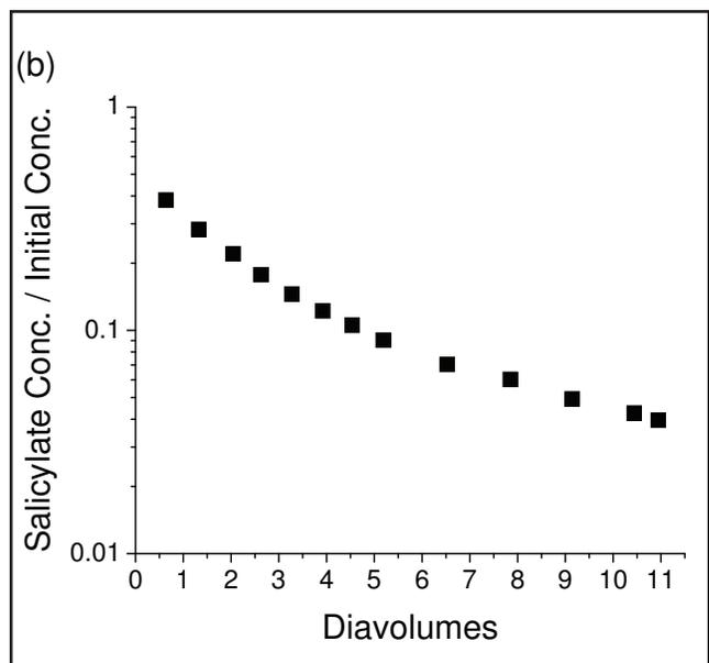
**Figures 7.** (a) Concentration of sodium salicylate leaving the permeate line when no BSA is present (control experiment). (b) Concentration of sodium salicylate impurity as it is removed from the BSA solution via diafiltration. The non-linearity shows the binding interaction that occurs between sodium salicylate and BSA.
