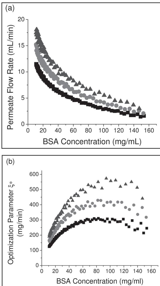
**Figures 5.** Permeate flow rate (a) and optimization parameter  $\xi^*$  (b) vs. BSA concentration at  $Q_{\text{feed}} = \blacksquare$  100 mL/min |  $\bullet$  200 mL/min |  $\blacktriangle$  300 mL/min at  $P = 20$  psi. High crossflow rates allow for higher permeate fluxes at the same BSA concentration and thus, higher  $\xi^*$ .
