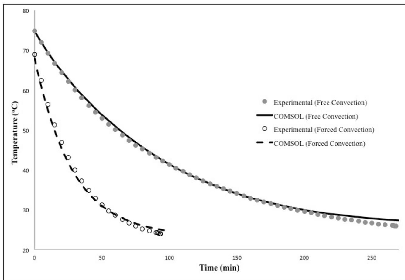
**Figure 2.** Temperature profile for aluminum cylinder at centerline radial position. Free and forced convection experimental data as symbols and COMSOL results as curves.
