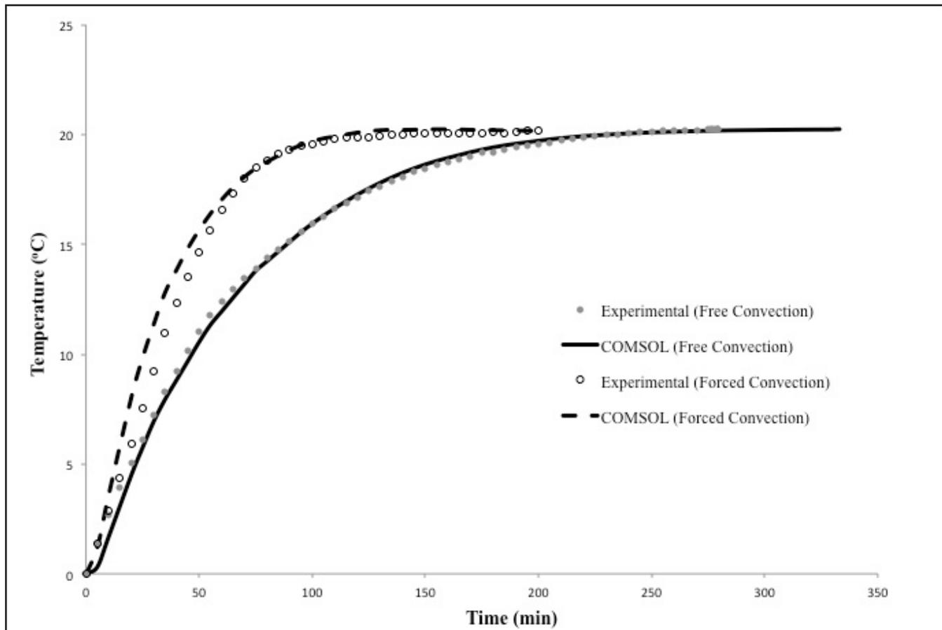
**Figure 3.** Temperature profile for the water balloon at the center position. Free and forced convection experimental data as symbols and COMSOL results as curves.
