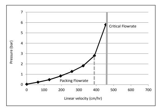
**Figure 4.** Pressure-flow curve to determine packing flow rate. The critical flow rate, defined as the flow rate at which the slope becomes infinite, was measured as approximately 450 cm/hr; higher linear velocities could not be achieved due to pressure limitations of the column. The packing flow rate is calculated as 85% of the critical flow rate.<sup>[16]</sup>
