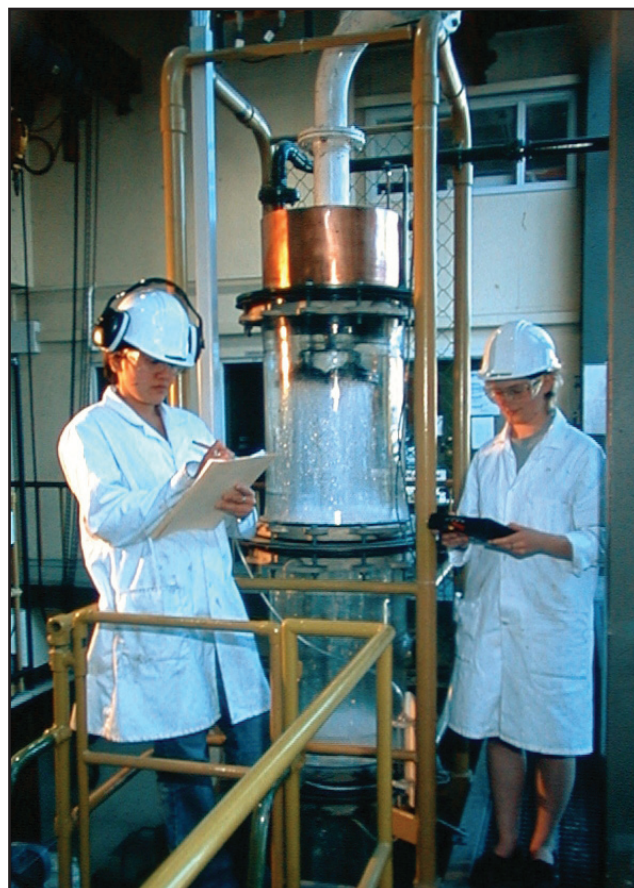
The 18" gas-liquid contactor used in the teaching lab.
