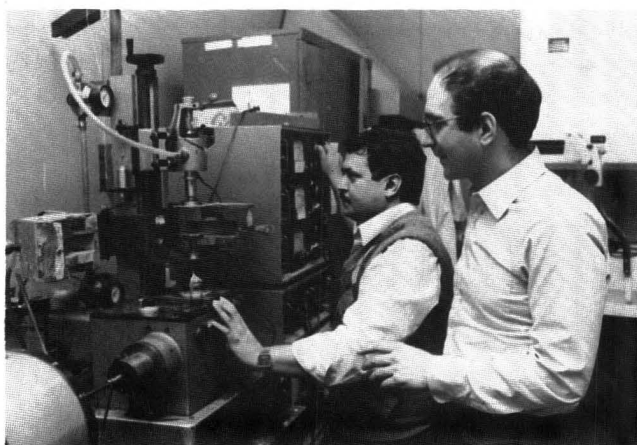
Taha Alkhamis and Richard Beissinger working with a Weissenberg rheogoniometer for blood viscosity measurement.
