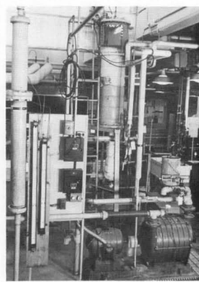
FIGURE 5. Air-water contacting in a spray tower. (a) Humidification, water cooling and dehumidification operations, and (b) effect of air and water rates on heat and mass transfer coefficients.
