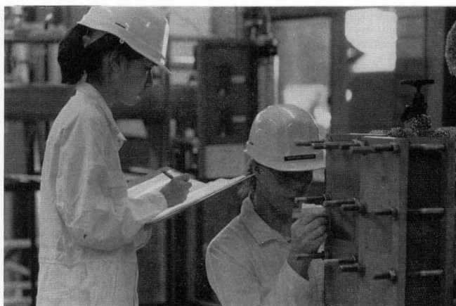
Students measuring spacings of plates on the plate heat exchanger.
