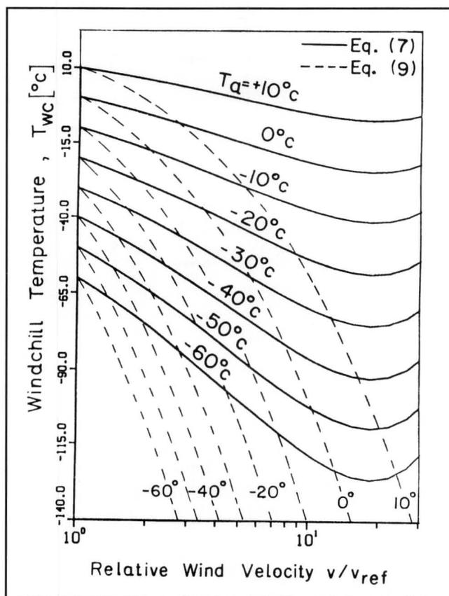
**Figure 3.** Wind-chill equivalent temperature versus wind velocity and ambient temperature.
