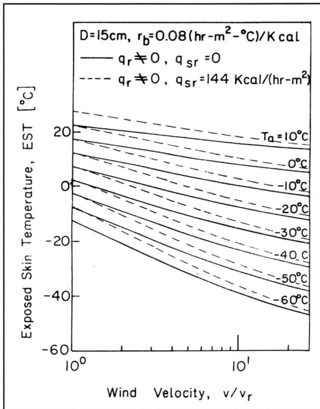
**Figure 4.** Exposed skin temperature with and without solar radiation.
