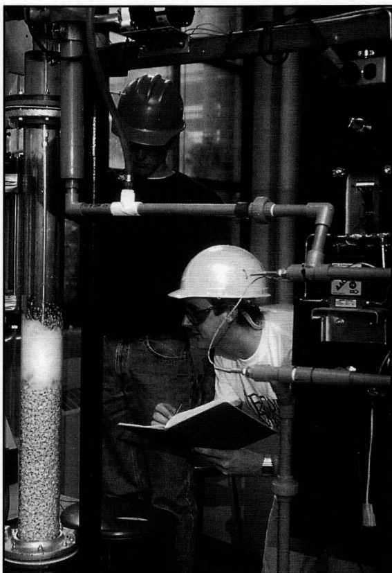
Marc VanderSchale and Brian Erickson remove CO 2 from air in packed-column gas absorber.
