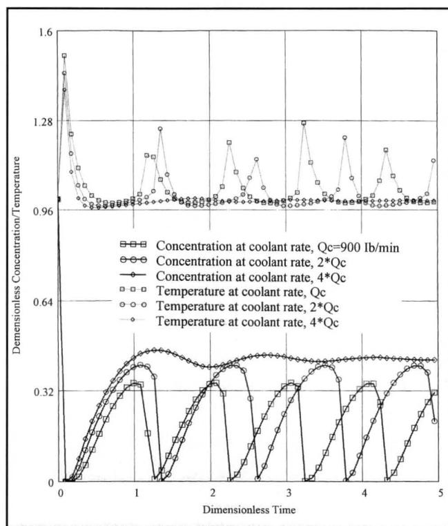
**Figure 4.** Case Study V: The effects of multiple-fold increase in flowrate of the coolant is marked by decreased frequency in oscillatory behavior of temperature and concentration, which eventually led to the disappearance of oscillation completely.
