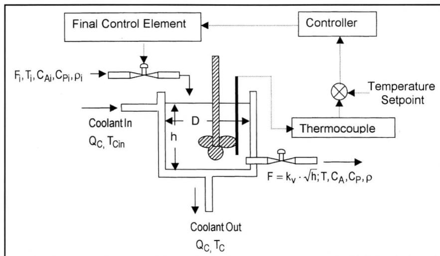
**Figure 1.** A closed feedback control loop of the modeled CSTR showing the essential components and parameters.
