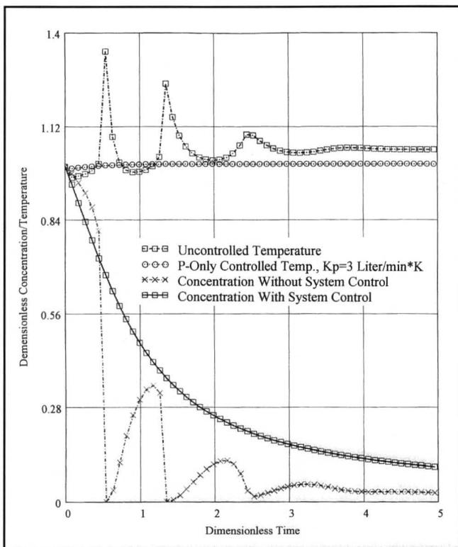
**Figure 3.** Comparison of Case Studies I (uncontrolled) and III (controlled) for temperature and concentration dynamics. Application of proportional control effectively removed the oscillations in both variables.
