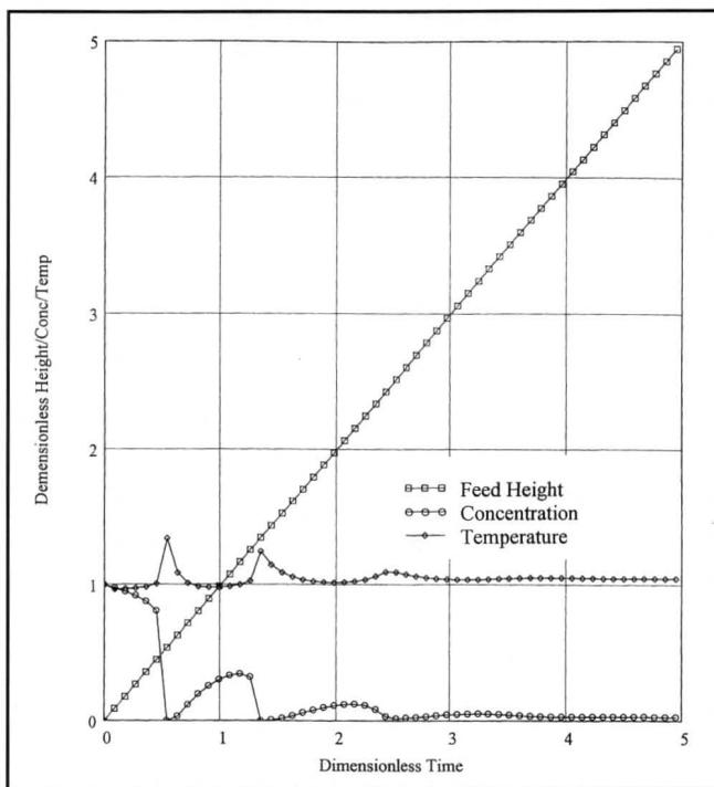
**Figure 2.** Case Study I: The dynamic response of the uncontrolled system during startup, with no effluent output. The tank fills at dimensionless time=1.
