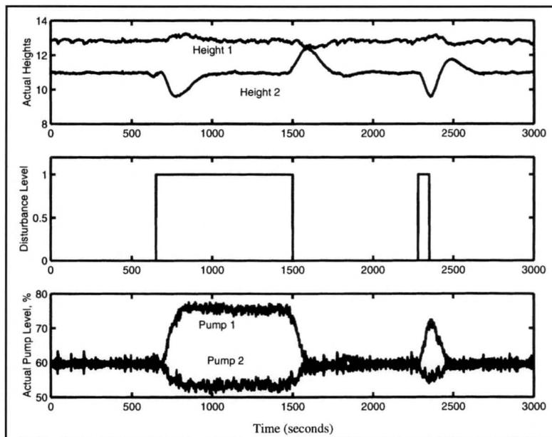
Figure 7. Disturbance rejection using robust controller.
