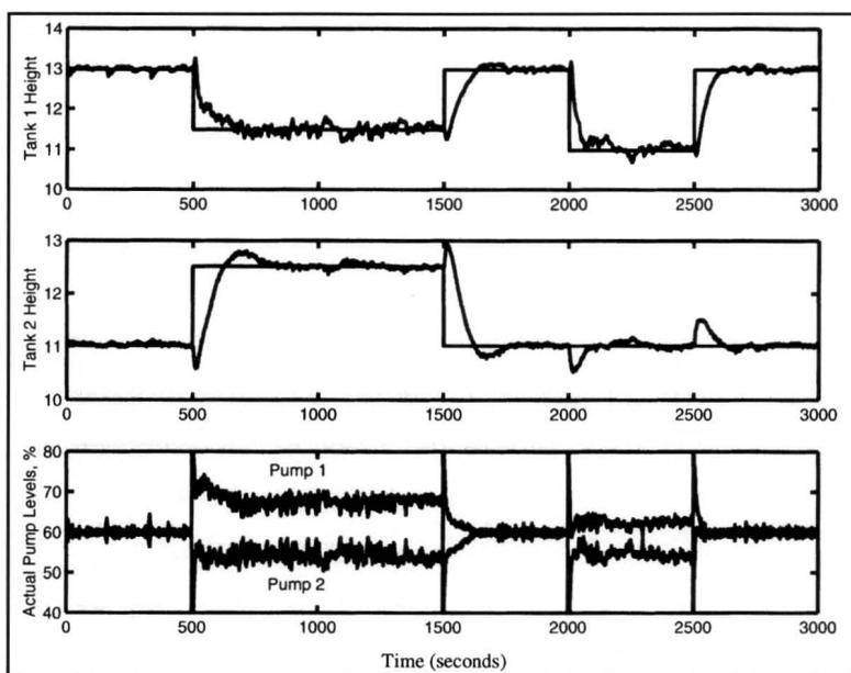
Figure 8. Reference tracking using robust controller.
