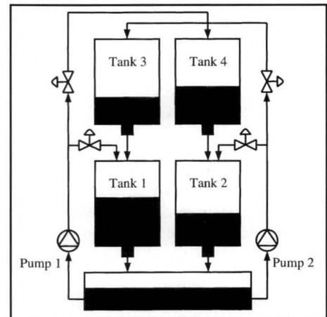
Figure 1. Schematic of the four-tank system.
