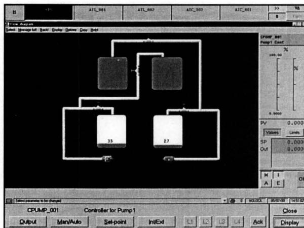
Figure 4. Screenshot of Freelance four-tank schematic.
