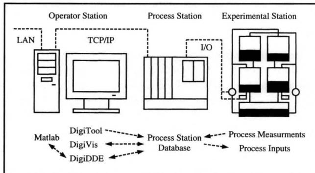
Figure 3. Schematic of the control system.
