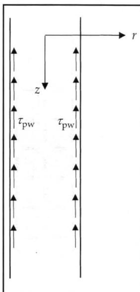
Figure 11. Coordinate system for one-dimensional standpipe flow.
