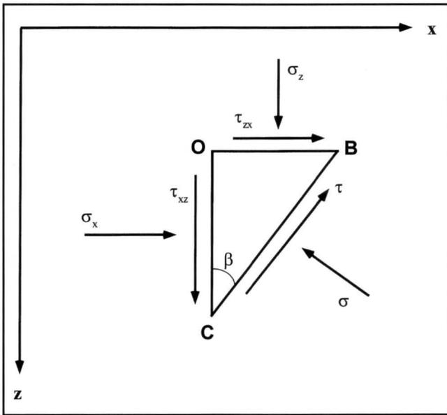
Figure 8. Equilibrium of stress components on a differential element.
