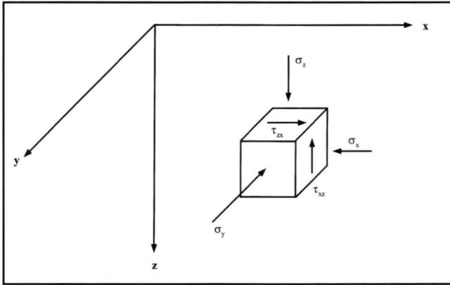
Figure 7. Stress components in a plane-strain problem in the x-z plane.
