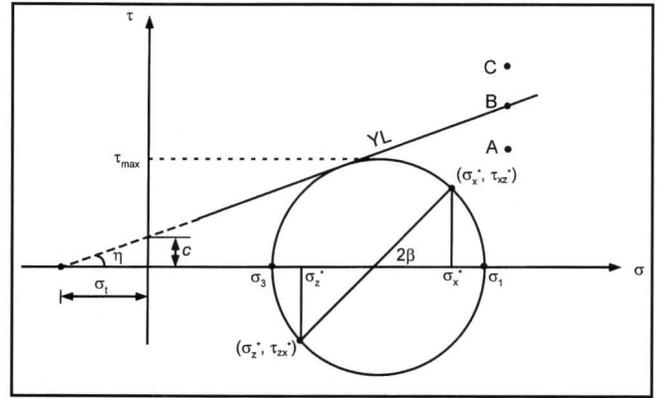
Figure 9. Mohr circle and Mohr-Coulomb failure envelope.
