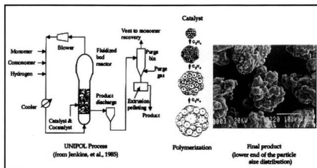
**Figure 2.** Chemical synthesis for the production of polyethylene/polyolefin (UNIPOL process).
