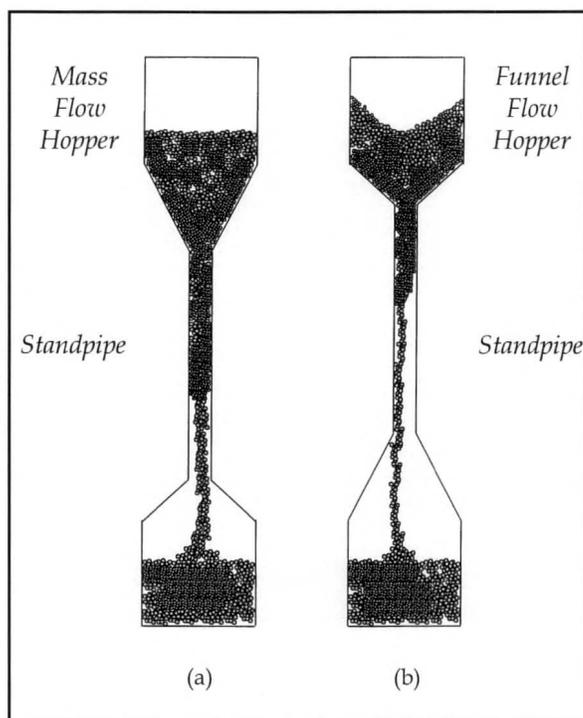
Figure 6. A device showing mass-hopper flow, funnel-hopper flow, and standpipe flow.
