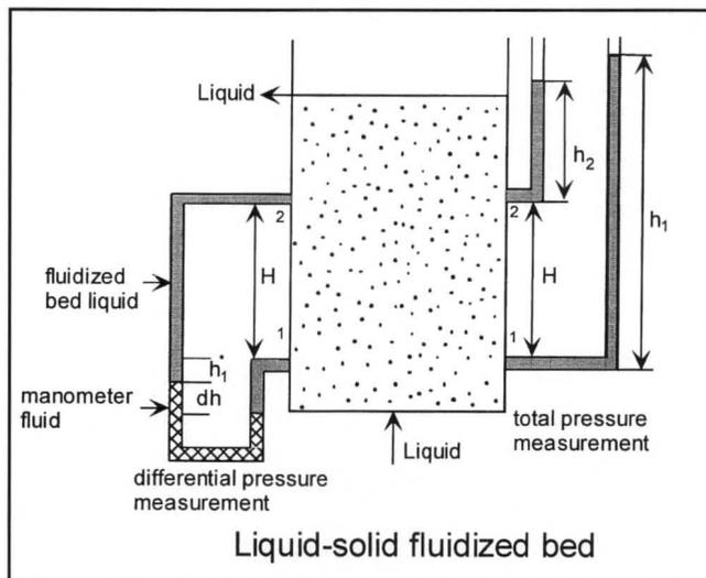
**Figure 3.** Pressure-drop measurement for a liquid-solid fluidized bed.
