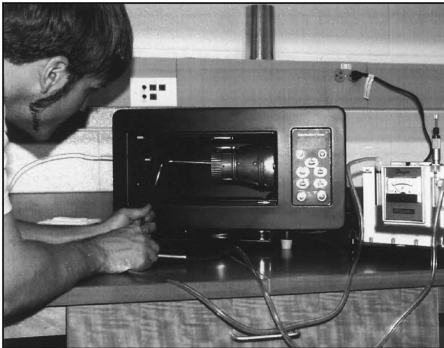
Figure 4. Student measurement of air velocity in a convection oven.
